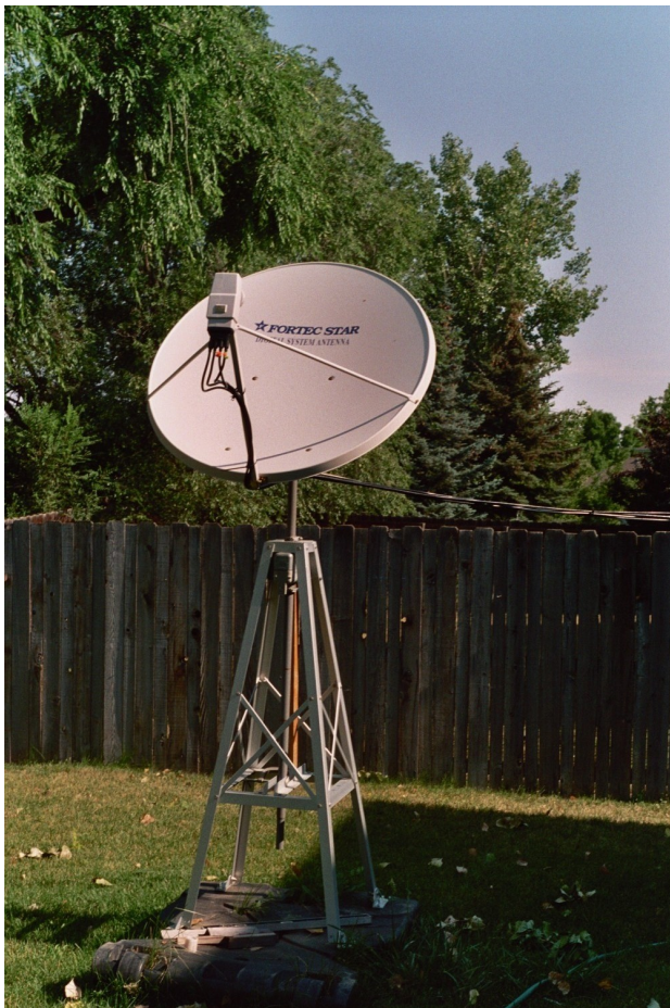
Illustration 1: A 90 centimeter offset dish with Invacom QPH-031 dual polarity dual frequency LNB.
