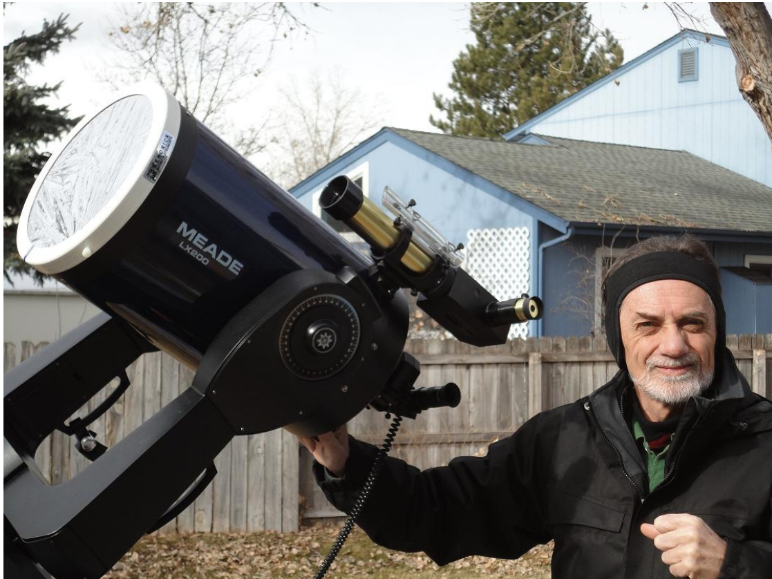
Figure 6, Rodney using a Baader white filter on a 10" Meade to count the sunspots. The long term goal will be to compare the SFI from the 2.8 GHz horn with the sunspot counts during this upcoming solar cycle 24.
